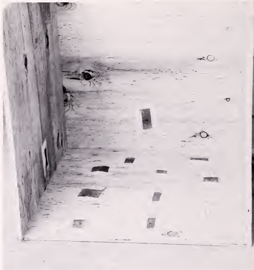
Forcing box with several breathing and drainage holes. The box is 2 ft. x 2 ft. x 2 ft. The holes are covered by window screen to prevent sand from spilling.
